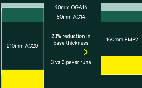
Diagram 1: Comparison between the typical pavement design for dense graded and EME2 asphalt base courses
