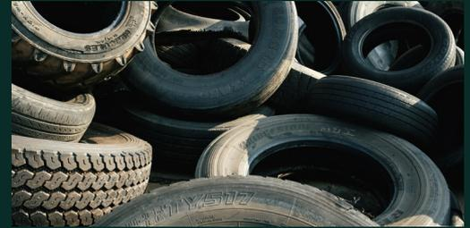
The use of crumb rubber modified DGA will provide a wearing or base course which will be less prone to cracking and rutting, more durable and require less maintenance during its service life.
